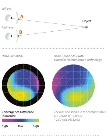
Figure 16: Comparison Convergence Difference (binocular)
