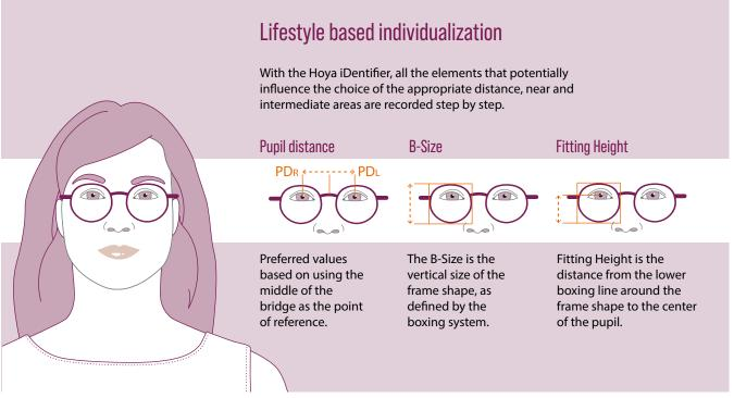
Figure 5: Pupil Distance, B-Size and Fitting Height
